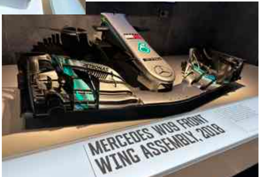
8: The front wing of the 2018 Mercedes W09
