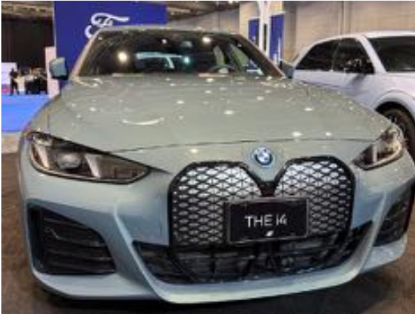
The BMW i4 is the AJAC Electric Car of the Year. The front grill is completely fake, but the outline can be illuminated.
