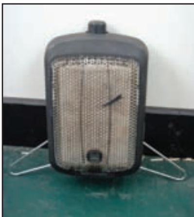
The small heater, showing where the rubber hose met the heat, and melted!
