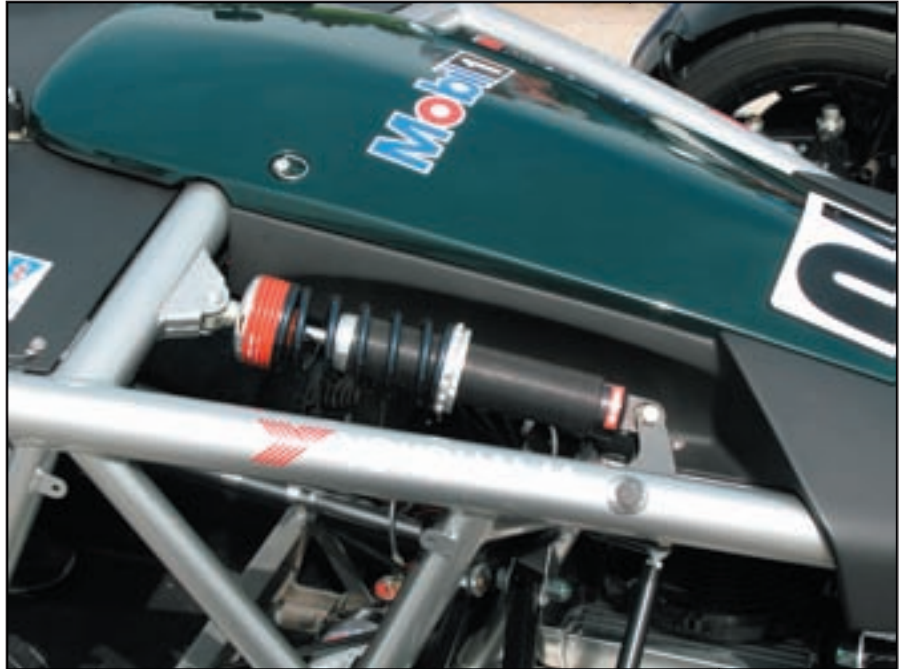
The push-rod front suspension on the Ariel Atom is definitely trick!
